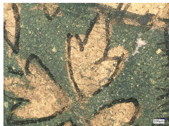
**Fig. 16** Large yellow crystals of orpiment are visible in the mixture of indigo and orpiment used for the majority of the green in this manuscript from 14th century Tabriz (Table 1, #8)
